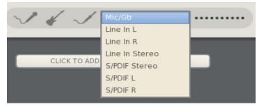
*Note: if you use the S/PDIF input, you MUST choose S/PDIF external clock option from the"Audio…" menu in the SETUP tab. Failure to do so will result in audio clicks and pops caused by errors in the data stream. By definition, digital audio inputs must have a corresonding clock source to keep the audio properly synchronized and free from data dropouts.*
