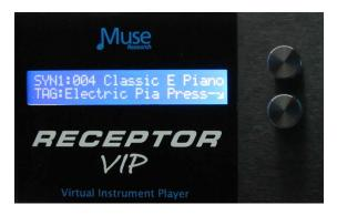
3. Now we'll layer that with another sound—say a pad synthesizer. To do this, we press the CHANNEL + button, and then the bottom encoder switch to add a new channel to what we already have loaded.
