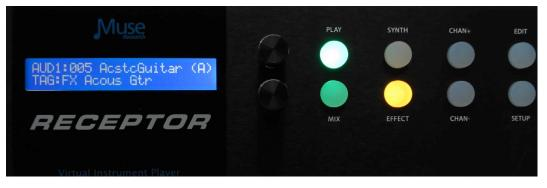
4. Bring up the gain adjacent to the front panel input, and verify that the input is not clipping when playing at your loudest level - the LED level indicator should never be red.
