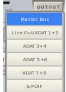
You can select more than one output at once, so you can have a channel go to the Master Mix bus as well as to any or all of the other physical outputs simultaneously.
