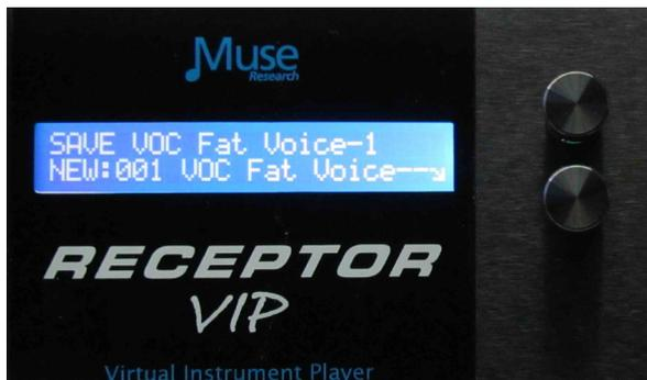
Simply use the bottom knob to select the location you want to save, and then press the bottom encoder to either create (if "new") or save (if writing over) the preset. Writing a preset takes a moment, after which time it will say "Created" on the display. All naming is automatic, but if you want to give them specific names you can do so using the Graphical User Interface.
