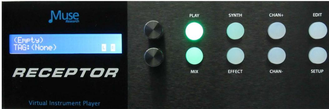
2. Next, we press the PLAY button and then select EFFECT channel. Since nothing has been loaded, we need to open up a channel which is done by pressing the bottom encoder.
