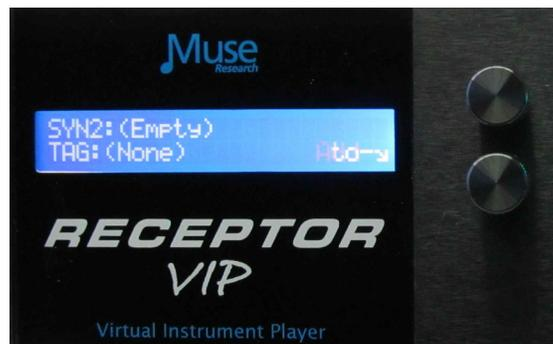
4. Select the TAG and preset of interest, say "Airy Pad" from the "TAG:Synth Pads" category. Press the knob to load this preset. Now press the "PLAY" button to hear both sounds combined together. What we've done is layered the Electric Piano and the Pad sounds together, which creates an entirely new sound. You can adjust the volume of either sound by pressing MIX and selecting the channel of interest to adjust the Electric Piano or Pad volume levels respectively.
