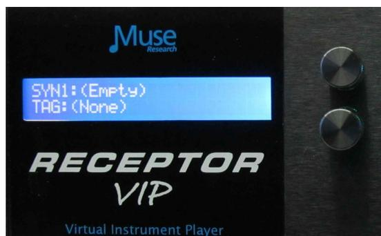
3. Now let's select a preset for this synth channel. Turn the bottom knob to find the sound you want. For example, let's choose an Electric Piano patch from the "TAG: Electric Pianos." Press the knob to load it
